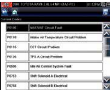
Read and clear OEM proprietary and global codes in just seconds with clear code definitions on screen.
