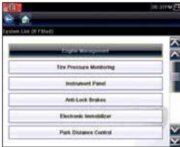
OEM-specific codes and live data graphing for critical vehicle systems.
