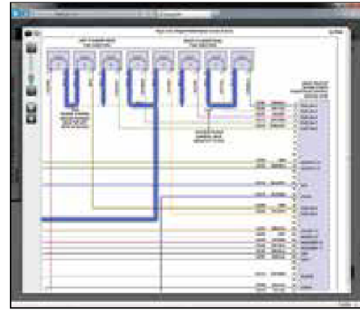
Full-color wiring diagrams with circuit highlights and zoom feature clarify even the most complex circuits.
